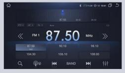
Supports "TA" and "AF" functions, the AF can search others transmitting frequencies automatically on current radio stations .and TA can search the same type radio stations automatically. Press "PTY" to allow the user to search their favorite program, such as specific types of music.
